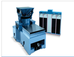
Composite Vibration Test System (11 ton)
