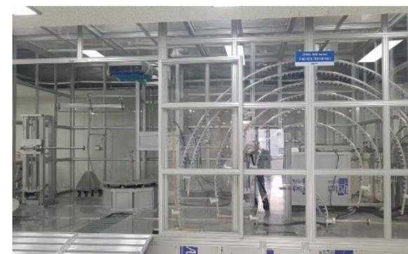
IP Tester, Dust Tester, UL 50E
